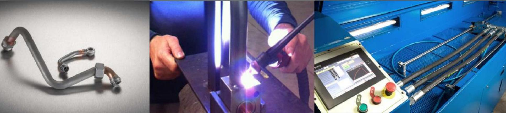
The welding of carbon and stainless steel is carried out by Strong brazing with filler material, Brazing in controlled atmosphere, MIG/TIG electrical welding granting to have complete flow of manufacturing process up to final bench test.
